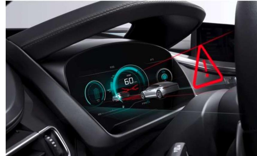
3D Display: allows the driver to take in the information faster than if it were displayed on conventional screens
