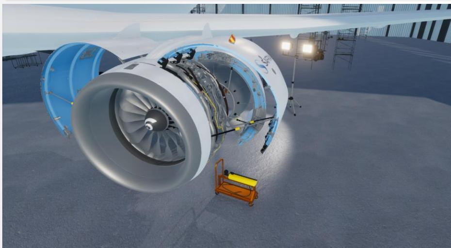
Release the rear HOR from the RRing on the engine.
